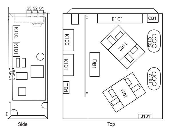
Figure 46. P300MT Component Identification
